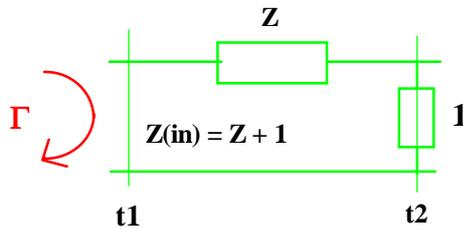
$$\Gamma = \frac{Z_{(in)} - Z_0}{Z_{(in)} + Z_0} = \frac{Z_{(in)} - 1}{Z_{(in)} + 1} = \frac{z + 1 - 1}{z + 1 + 1} = \frac{z}{z + 2} = S_{11}$$
