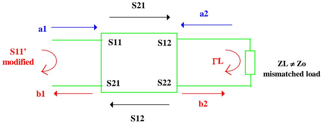
$$\Gamma_L = \frac{Z_L - Z_o}{Z_L + Z_o} \quad \Gamma_L = \frac{a_2}{b_2} \quad \therefore a_2 = b_2 \cdot \Gamma_L$$
