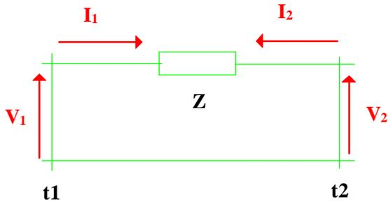
$$\left. \begin{array}{ll} V_1 = a_1 + b_1 & V_2 = a_2 + b_2 \\ I_1 = a_1 - b_1 & I_2 = a_2 - b_2 \end{array} \right\} \text{General}$$
