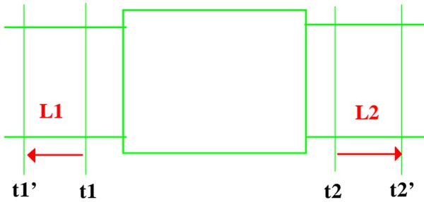
Note positive signs for L1 & L2 are taken to be movements away from the device
