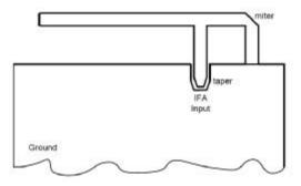
• The miter is used to avoid a right angle microstrip bend, which results in a poor current flow on the stub.
