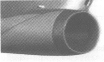
图 2 某型无人机吊挂式进气道 Fig. 2 A hanged duct of pilotless aircraft
