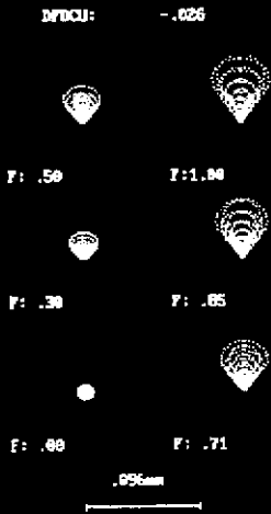
Fig.4 Spot diagram of Cassegrain system
