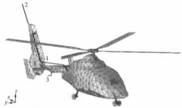
图 1 直升机实体模型与表面网格剖分效果 Fig. 1 The full size helicopter model and its surface meshes
