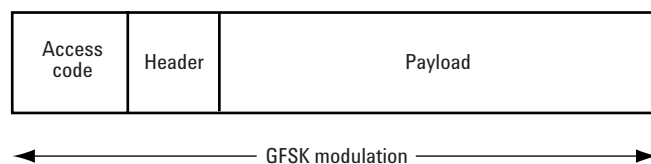
Figure 3. Bluetooth basic rate packet format
