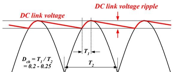
Figure 2. DC Link Voltage Waveform
