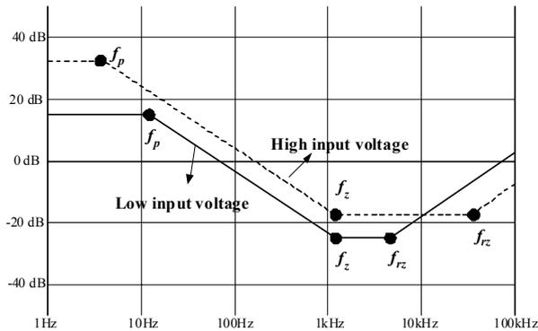
Figure 7. CCM flyback converter control-to output transfer function variation according to the input voltage
