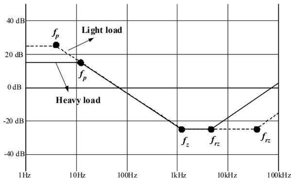
Figure 8. CCM flyback converter control-to output transfer function variation according to the load
