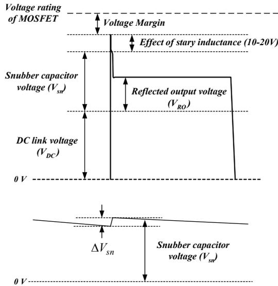
Figure 5. MOSFET voltage and snubber capacitor voltage
