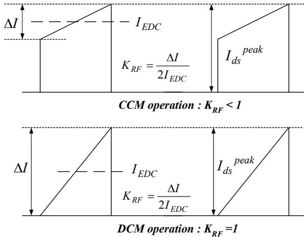
Figure 3. MOSFET Drain Current and Ripple Factor( $K_{RF}$ )
