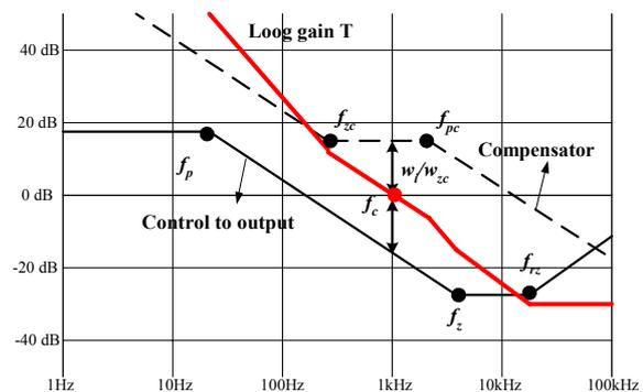
Figure 10. Compensator design
