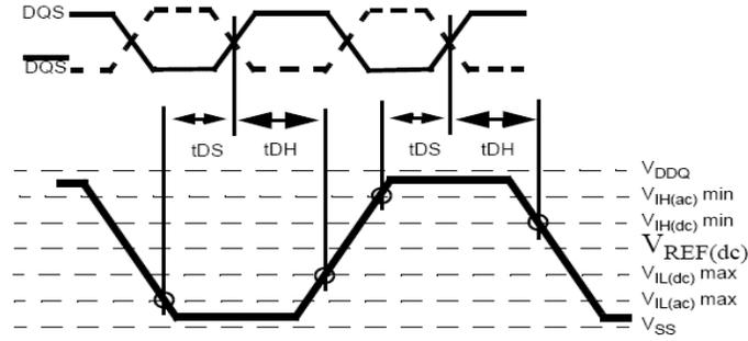
Figure 90 — Differential input waveform timing – tDS and tDH
