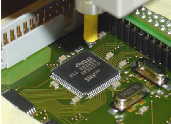
Figure 4: Surface scan setup (IC with H-field probe).
