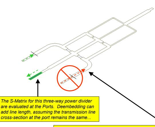
...subtracting length is also possible. However, specifying a distance which would deembed past a **change** in the transmission line cross-section will provide invalid results!!
